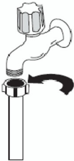
Figure 5- Connecting the supply hose to a \frac{3}{4} inch tap.
